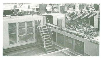
Shipped to Pontiac Motor Division, G.M.C., last week was this Wheelabrator Ram Tunnel Blast Machine. It will be used to clean automotive head castings at the rate of 1200 per hour — that's one casting every three seconds. The heads are automatically loaded onto a loading conveyor (right foreground) and then rammed into the blast tunnel. The abrasive blast from nine blast wheels removes all the molding sand.
